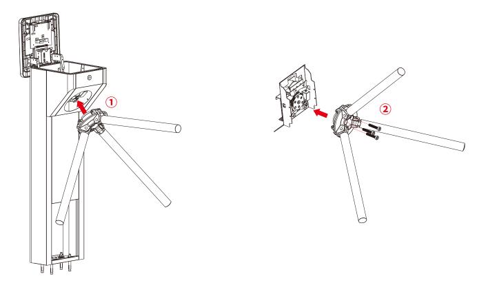
11. After assembling the arm, the resistance of the arm can be adjusted by rotating the damper left and right. Rotate the damper and observe the number on the damper. The greater the number it is, the larger the resistance will be.
