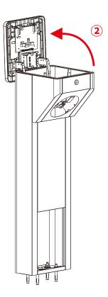
10. Align the arm assembly with the assembly inside the chassis, and then secure it with screws.
