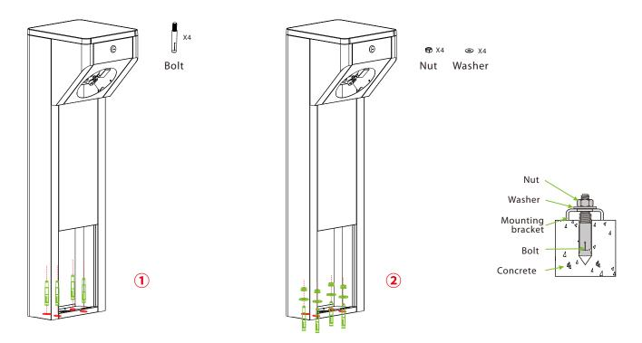
**Note:** Before inserting the bolt, the user must pull the power cable and Ethernet from the machines and put them into the wire slot.
